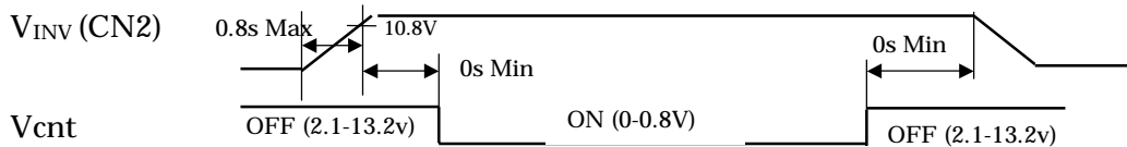
Figure 10-4 Power Supply Sequence(Inverter)
